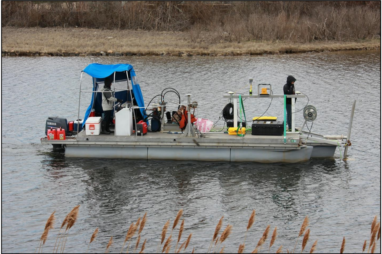
Figure 5: The 28' pontoon-type vessel that will be used for the surveying work.
